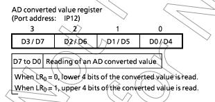
Figure 3-19. AD converted value register
