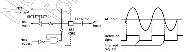
Figure 3-24. Zero-cross Detector
