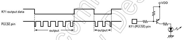
Figure 3-23. Circuit Example of Carrier Pulse and Timing
