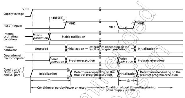
Figure 3-32. Port condition by Reset operation
